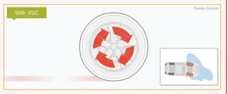
For example, if your ESC system detects a case of over-steering, it will automatically apply the front outside brake to counter the loss of traction affecting the rear wheels. In the case of under-steering, ESC will apply the inside rear brake, encouraging the vehicle to continue to turn in the direction indicated by the driver's steering input.
