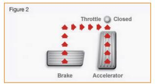
safely bringing the vehicle to a stop. To illustrate, brake override can detect if the driver is pushing the accelerator and the brake at the same time. The safety system recognizes this is not how people normally drive, and proceeds to initiate corrective action. Brake override is designed to override accelerator commands when appropriate, and will not override the brake.
