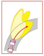
Adaptive headlights can redirect beams toward the direction your vehicle is turning.
