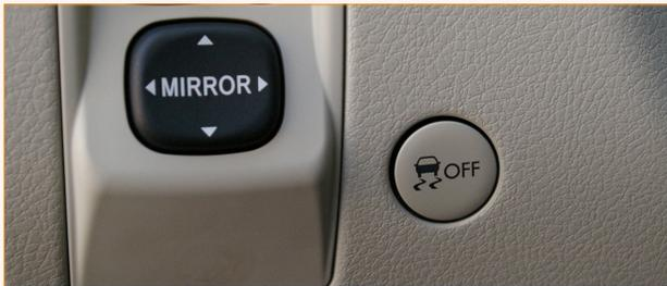
Most manufacturers install a button that allows drivers to turn ESC off. When you turn off ESC, the traction control component of the ESC system will deactivate. This would be helpful if, for example, you were driving in deep snow, mud, or sand; you were driving with chains on the tires; or, you were driving using the spare tire (Transport Canada 2012).
